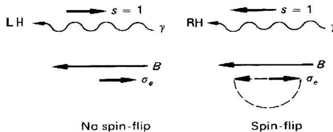
**Figure 5:** Compton scattering by polarized atomic electrons. The case where the photon cannot be absorbed is shown at the left and the case where the photon can be absorbed by flipping the spin is shown to the right.
